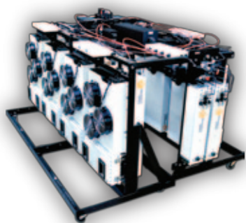
Modular design with built in redundancy 3K Ku-band System GaN Based - SapphireBlu™ Series
