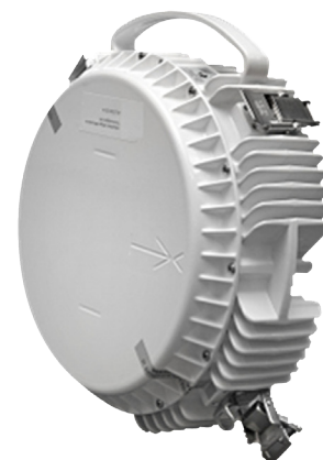
Common outdoor unit (ODU) for microwave radios
