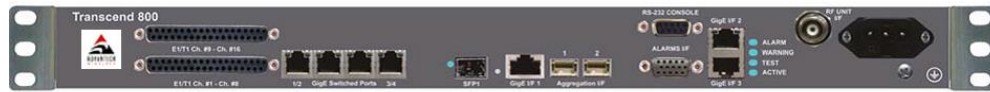
Transcend 800 Indoor Unit (IDU) Version with interface for 1xSTM-1/OC-3, 16 E1/T1 & 7 GigE interface
